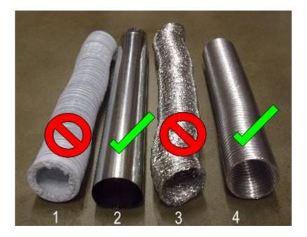
Albert Lea Fire Rescue would like to remind you to use the correct type of dryer vents to help prevent fires. See in the picture that Vent #1 and Vent #3 *are not allowed* per Minnesota State Mechanical Code; these are Flexible and Vinyl style dryer vents.
