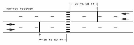
Figure 3 – Stop Line Markings
