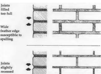
Left: Historic photo of First National Bank Building, note the masonry detailing. (Albert Lea Tribune) Right: Comparison of the effect of mortar installation methods. When joints are filled too full, it changes the character of the brick wall. Most historic joints are slightly recessed. Repointing work should match the historic condition as close as possible. Image courtesy of the National Park Service (Preservation Brief 2: Repointing Mortar Joints in Historic Masonry Buildings).
